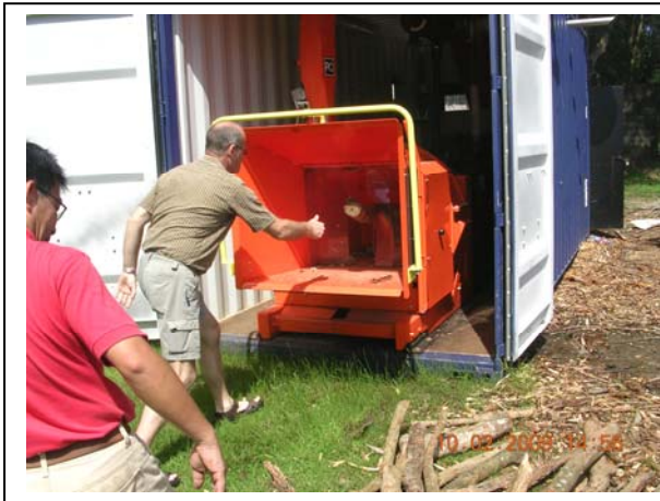
Container with Chipper, 120 kW diesel engine and Briquetting Machine
