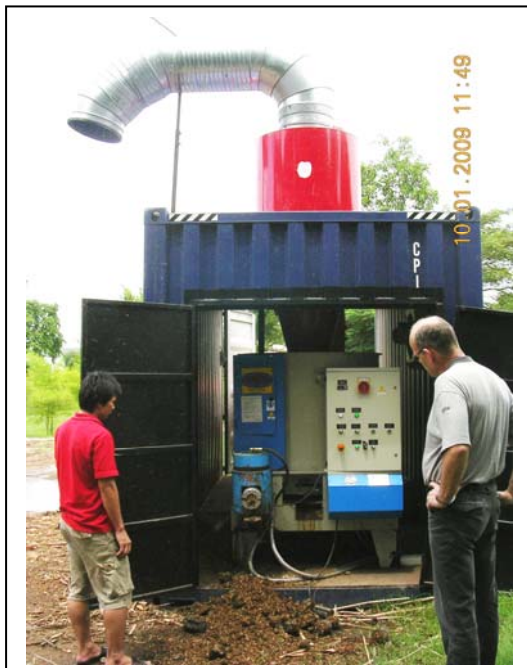
Container with Chipper, 120 kW diesel engine and Briquetting Machine
