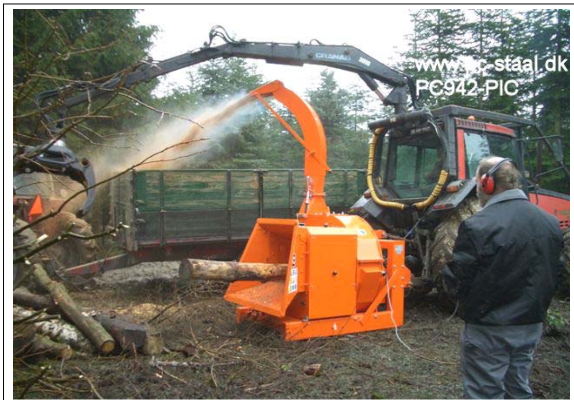
The maximum tree/trunk diameter that can be accepted is 27 cm/ 10.3 inch
