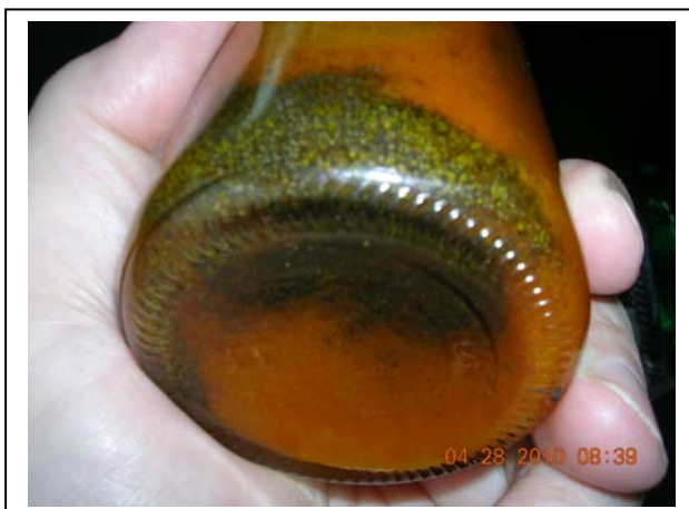
The above pictures show oil samples, left at the test site overnight, samples taken on April 27. The black fiber is most probably coming from the decanters; the efficiency of the decanters seems to be slightly reduced at full load. Biomass fiber is known to be very good to soak up oil, and is commonly used in connection with oil spill. It is believed that the fiber content in the POME will soak oil that is then discharged together with effluent from the MORE test unit.
