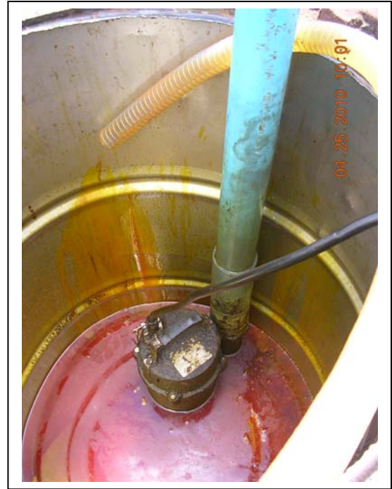
The oil being recovered during the morning of April 25 later proved to have an FFA % of 5.71 % and the impurities were as low as 0.07 %. Unfortunately the oil loss in the effluent from the test unit was not measured
