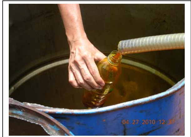
Oil sampling for visual inspection
