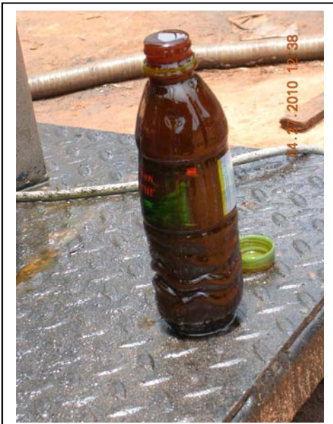
Inaccuracy in the sampling of POME from the pit, resulted in the mounting of a sampling valve and a small hose at the test unit pump (outlet was higher than inlet)
