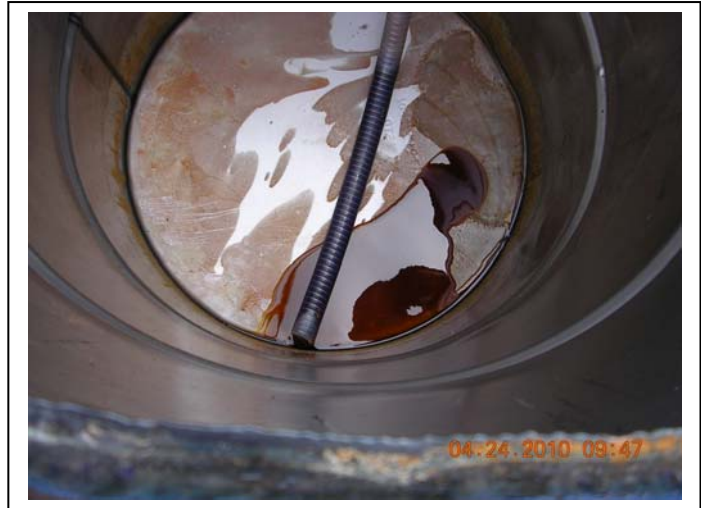
Right after the incident with overflow from the pretreatment tank the first recovered oil started to flow from the test unit
