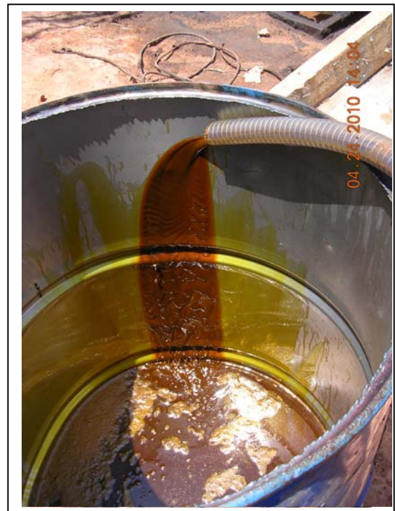
The oil recovered during the afternoon of April 24, the first day of testing the oil recovery unit. Note the relatively dark color of the recovered oil. The dark color indicates that this is not fresh CPO.
