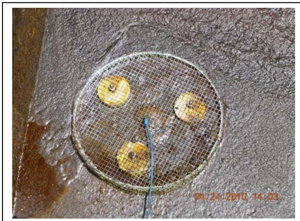
The oil recovered during the afternoon of April 24, the first day of testing the oil recovery unit. Note the relatively dark color of the recovered oil. The dark color indicates that this is not fresh CPO.
